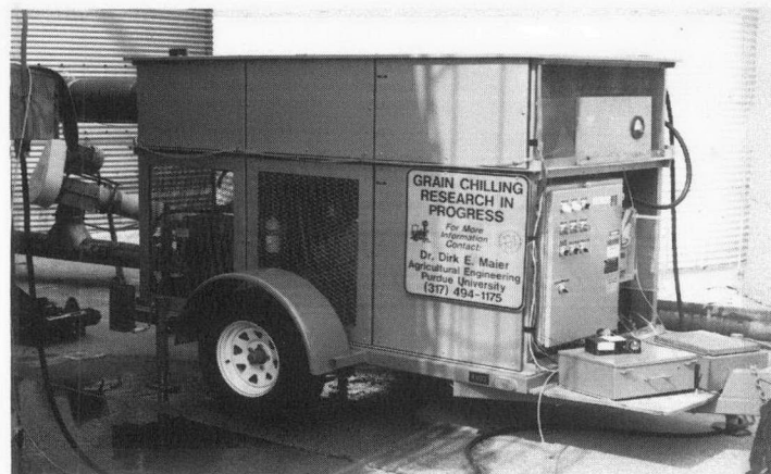
Fig. 6. Prototype grain chiller developed jointly by Purdue University and AAG Manufacturing (Milwaukee, Wisconsin, USA) operating during the optimisation test runs in 1992.
