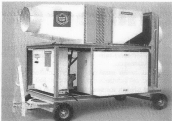
Fig. 2. Commercial grain chiller Granifrigor KK400 manufactured by Sulzer-Escher Wyss, Lindau, Germany.
