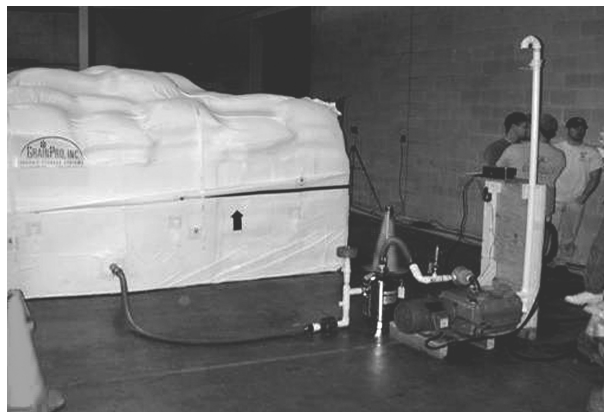
Figure 1. A V-HF Cocoon™ holding cocoa beans in bags, under a pressure of 50 mm Hg connected to the vacuum pump in a trial site in Boston, Massachusetts (courtesy of GrainPro Inc.).
