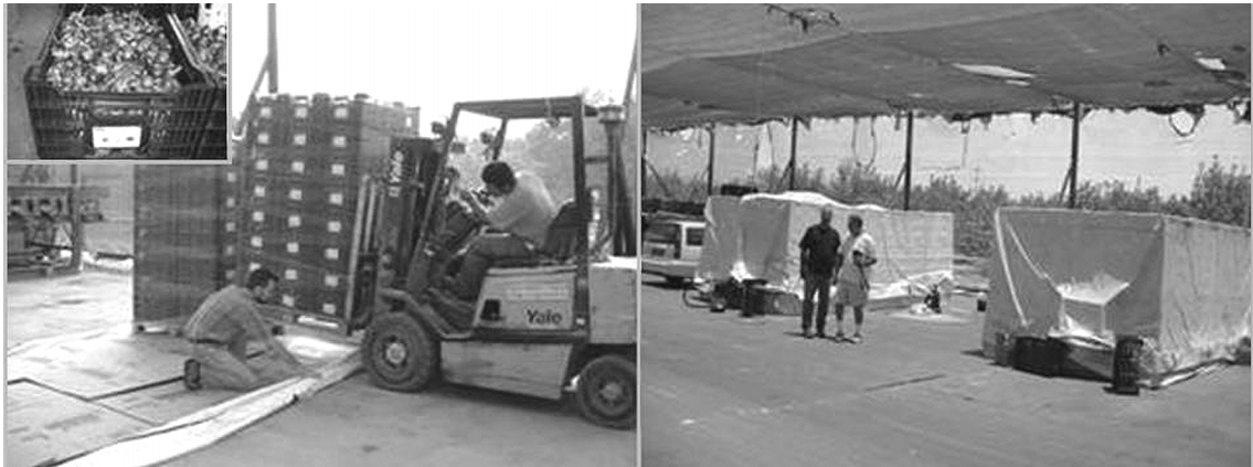
Figure 2. Narcissus bulbs in standard boxes before loading on pallets (upper left), loading the pallets containing the narcissus bulbs (left), and the general view of two sealed V-HF Cocoons™ under treatment (right) (courtesy of GrainPro Inc.).
